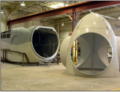
Hand lay-up offers low-cost tooling, simple processing and a wide range of part size potential. Design changes are made easily. Parts have one finished surface and require secondary trimming.
