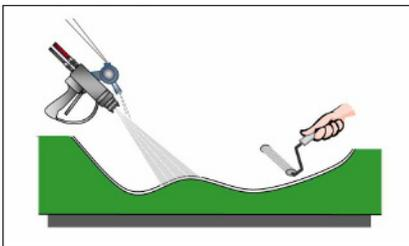
Similar to hand lay-up in simplicity, spray-up offers greater shape complexity and faster production. It too uses a low-cost open mold (one finished part surface), room temperature curing resin, and is suited for producing large FRP/Composite parts such as tub/shower units and vent hoods in low to moderate quantities. Cure is usually at room temperature, but can be accelerated by application of moderate heat.
