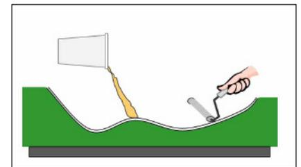
The simplest and oldest of the fabrication processes for FRP/Composites, hand lay-up, is used in low-volume production of large components such as boat hulls and associated parts.
